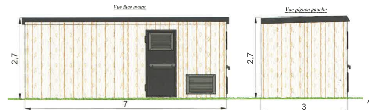
Figure 3 – Poste de transformation (dossier PC, UNITE)
