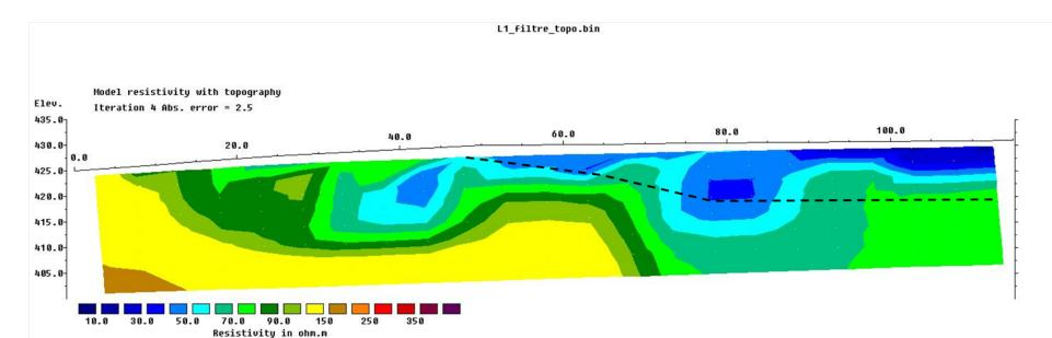
Horizontal scale is 57.50 pixels per unit spacing Vertical exaggeration in model section display = 0.63 First electrode is located at 0.0 m. Last electrode is located at 115.0 m. Unit Electrode Spacing = 5.00 m.
