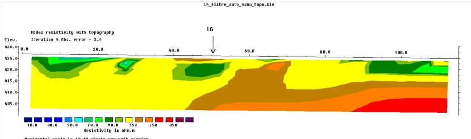
Horizontal scale is 60.00 pixels per unit spacing
